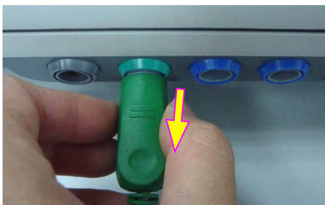
Disconnecting the transducer
