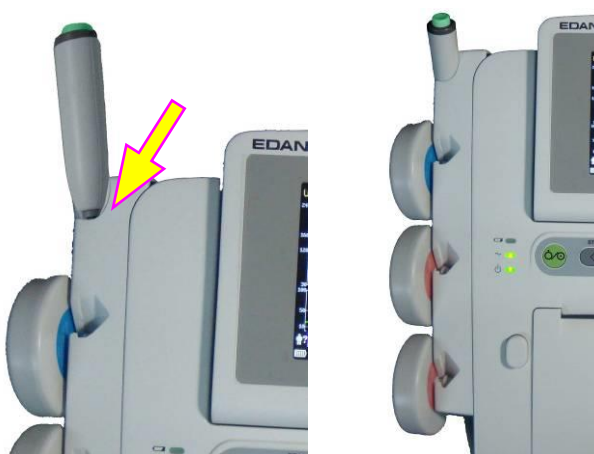
Placing the marker
